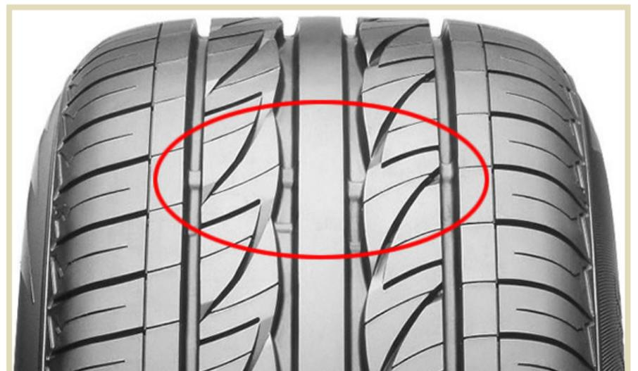
that it is wearing evenly. If one side of the tire is wearing faster than the other, you have problems with your car's alignment. If both outer edges are wearing faster than the middle of the tread, you are running your tires at too low a pressure. If there is more wear in the center of the tread than there is on the sides, you have been running your tires with too much air pressure.
