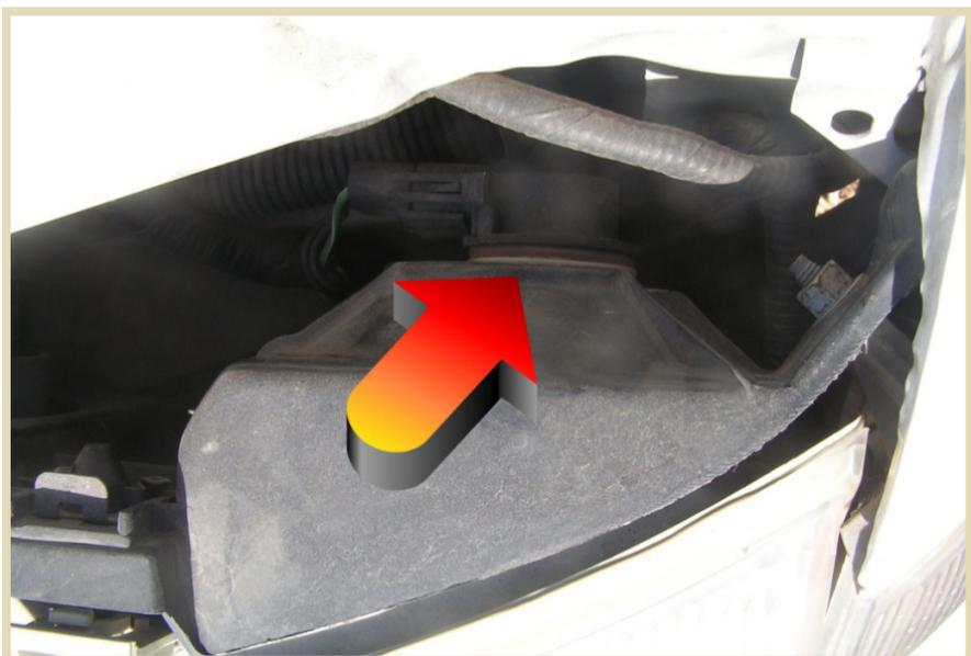
alignment of the socket in the light housing, as this will help you to reinstall it.
