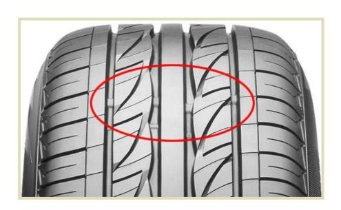
that it is wearing evenly. If one side of the tire is wearing faster than the other, you have problems with your car's alignment. If both outer edges are wearing faster than the middle of the tread, you are running your tires at too low a pressure. If there is more wear in the center of the tread than there is on the sides, you have been running your tires with too much air pressure.
