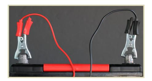
Car battery terminals tend to corrode over time. If this gets bad enough, the battery will no longer recharge or pass current to the engine so that it can start. Corrosion should be cleaned off with a wire brush and baking soda dissolved in water.
