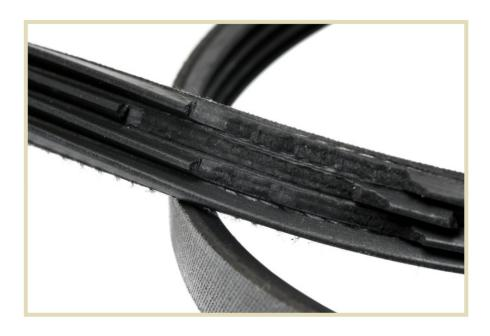
out of alignment. Likewise, excessive wear to the edges of the belt will indicate a pulley out of alignment.
